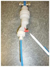
2. The device does not have the reset attached in which case you have to undo the reducer on the bottom of the water block and press in the red pin indicated.
